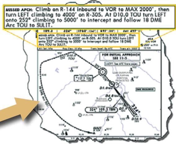
brief, the missed approach. We recommend that the Pilot Flying (PF) reads the missed approach from the MCDU, while the Pilot Non Flying (PNF) confirms by reading the missed approach section of the chart. Use of the ND in plan mode will give a good visual confirmation at the same time.
